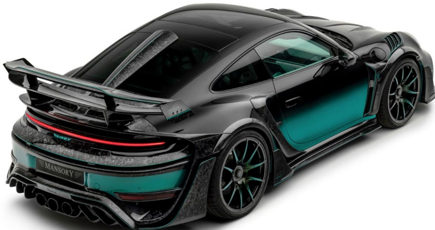
The air intakes in the rear side panel are framed by large air inlets made of visible carbon and, in conjunction with the additional intake scoop on the rear window, ensure that sufficient fresh air flows to the engine in every driving condition.
