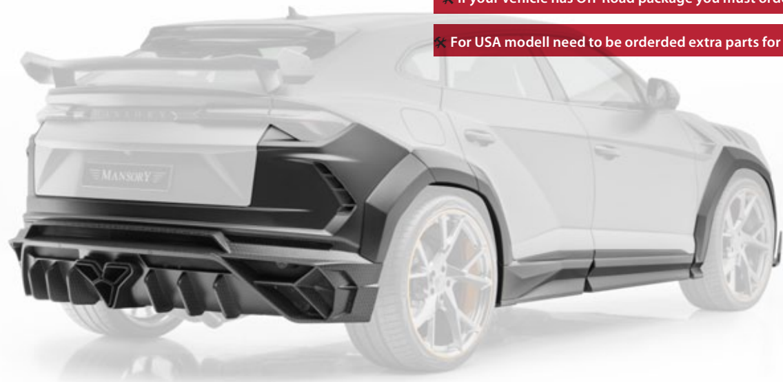
Long air outlet cover 636 802 501 for MANSORY wide body rear bumper visible carbon fibre primed without clear coat 2 parts set - left & right
